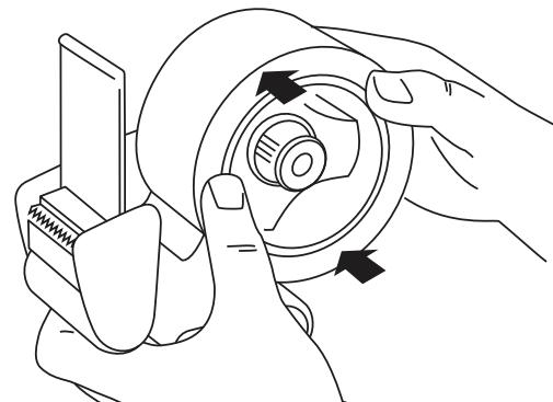
Insert the roll of packing tape onto the large dispenser wheel on the top-right of the tape dispenser with its handle grip to the right. Position the tape roll so that it will unwind with the sticky side facing down as the dispenser is pulled backwards.
