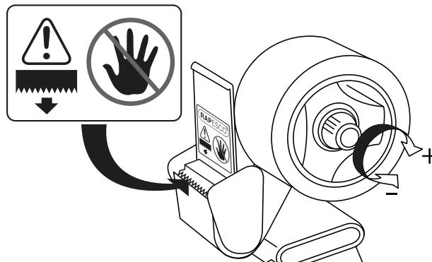
Adjust the tension on the dispenser (in the centre of the large dispenser wheel) to set a smooth and comfortable unwind mechanism.
