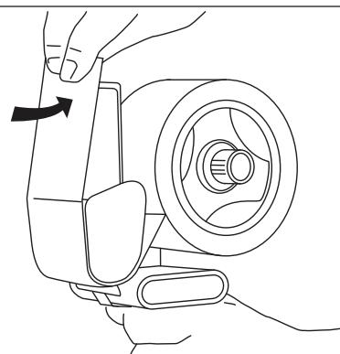
Pull up on the tape so the tape is over the cutting bar/ serrated blade, being careful not to cut yourself on the sharp blade.
