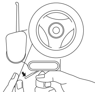
Pull the front end of the tape roll through the slot between the dispenser roller and metal guide. The guide can be held open by pressing down on the extended metal tab. The sticky side of the tape should face down/ away from the edge of the blade. If you have the tape in the wrong way, the tape will stick to the dispenser roller, so make sure the sticky side is face down.
